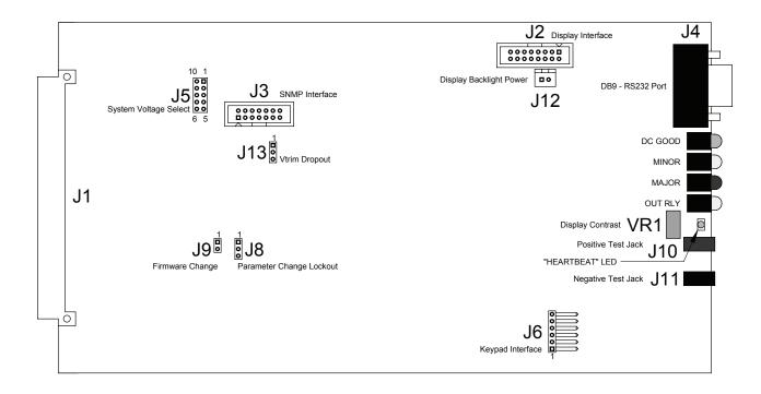
Figure 5.2-1 Controller Card Jumper Locations
